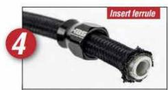
Push the aluminum ferrule onto the hose between the inner hose and the stainless/ cloth outer braid. Make sure the ferrule is pushed on the entire way. Pressing it against a flat surface once started can help.
