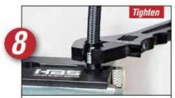
Using the 414-905 Aluminum AN Adjustable Wrench, tighten the nut down onto the body until there is less than 1/16" gap between the nut and the body.
