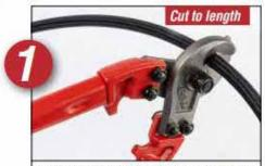
Use our 414-900 Hose Cutter to cut the hose to length. Alternatively, wrap with electrical tape at cutting point and use a very sharp fine tooth hacksaw.
