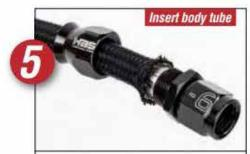
Insert the tube from the body of the fitting into the PTFE inner tube so that the shoulder of the body fits squarely against the femule.
