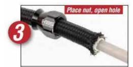
Slide on the nut in the direction shown. Remove tape if used during cutting. Use a round object (such as a pen or dowel) to make the inside of the line round. It can get deformed from cutting.
