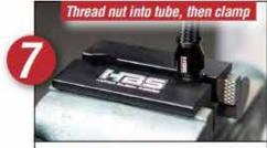
Pull the nut down over the outer braid and begin to thread the nut to the body by hand. Once the nut and body start to thread together, place body in aluminum vise jaws.
