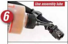
Place a drop of assembly lube onto the threads of the fitting body. The lube helps make assembly easier and keeps the threads from galling so that the fitting can be reused.
