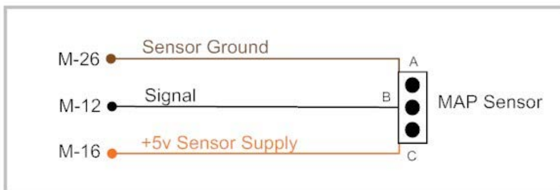
Manifold Absolute Pressure Sensor Wiring
