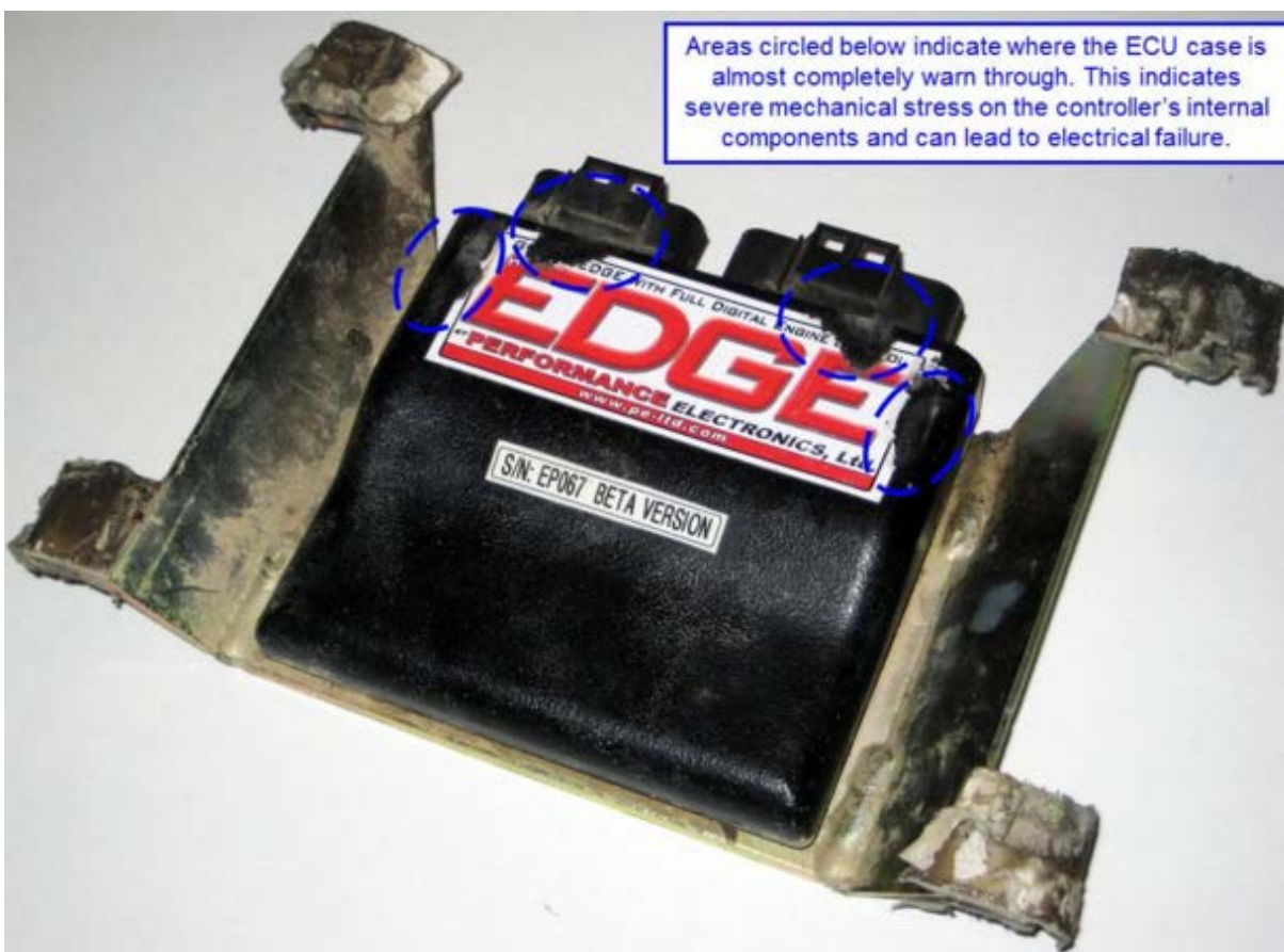
Mechanical Damage to the EC U Resulting in Premature Internal Failure
