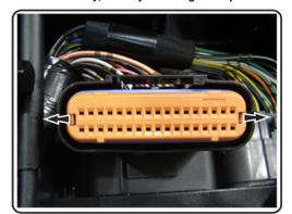
Insert a very small flat head screwdriver into the large hole above the contact that is to be removed. Gently pry up with the screwdriver to unlock the contact and pull on the wire to the contact from the rear of the plug to remove it.
