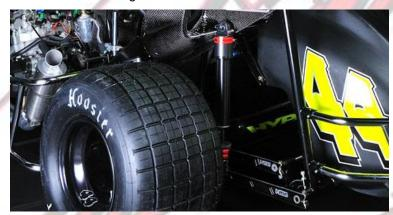
This picture shows the proper use of a left rear bump rubber. Use the shims to adjust exactly when the car gets into the bump rubber. Try to get the shock to hit the bump rubber about 3/4" before the frame hits the ground.
