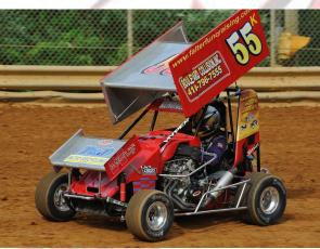
You can see in the above pictures that the cars are now transferring weight to the right side of the car in the rolled right phase on corner exit. Interesting too you can see in Robie's 55 car, the left front shock is topped out and just about off the ground, all the weight that was on the left front has now mostly transferred to the right rear and right front, He can still steer off the right front, so this is not a bad thing.
