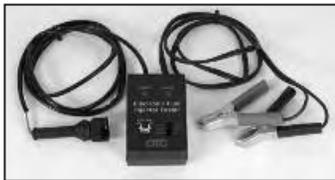
**Fuel Injector Pulse Tester**
