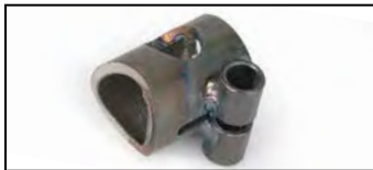
Socket Pinch Assembly uses 5/16"-24 x 1-1/2" long HHCS bolt with nylock full nut, not included.
