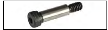
5/16"-18 Shoulder Bolt, for Electric Wing Adjuster Motor (each) Drill out the electric wing motor to 5/16" hole for this bolt to fit through. 5/16 x 7/8" long with 1/4-20 threads. 30-205 $3.45
