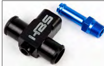
1" Inline Coolant Fitting, Oil Cooler and Mychron Water Temperature Sensor Designed for engines that have an external oil cooler (includes Yamaha and Suzuki 600cc) that needs to be T'd into the coolant line going from the head to the radiator. Inline fitting features 1" barbed ends, M10 x 1.00 port for the MyChron water temp sensor 604-201 and a 1/2" NPT port used for the oil cooler line. Choose 1/2" or 3/8" barbed to 1/2" NPT fitting.
