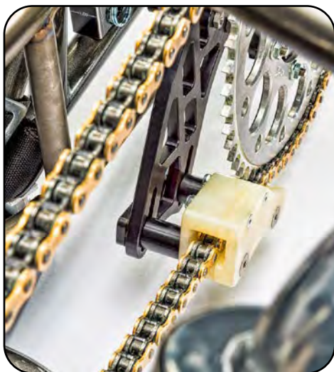
NYLON GUIDE BLOCK PREVENTS CHAIN SKIPPING
