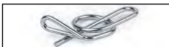
Heavy Duty Rue Clip for 1/2" Shock Stud New heavy duty rue clip has a thicker wire and a built-in handle for easy removal. Fits all of our new shock studs, but in older pins, the hole must be drilled out to .149" (#25 drill). 38-8024 $1.25
