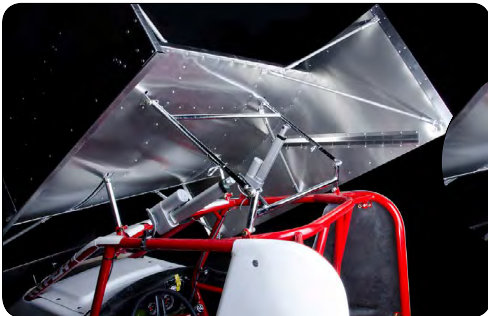
HYPER WINGS 12' SQUARE INTERNAL SLIDER WING WITH 54" SIDE PANELS AND DUAL WING ADJUSTER ASSEMBLY
