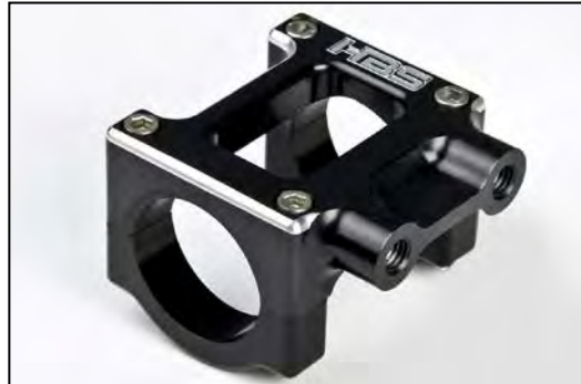
Axle Clamp for Steering Box Use with axle mounted box instead of welding bosses onto axle. 6061 T-6 aluminum. 16-525 1 1/2" AXLE $45.00 16-526 1 1/4" AXLE $45.00 16-527 1 3/4" AXLE $45.00
