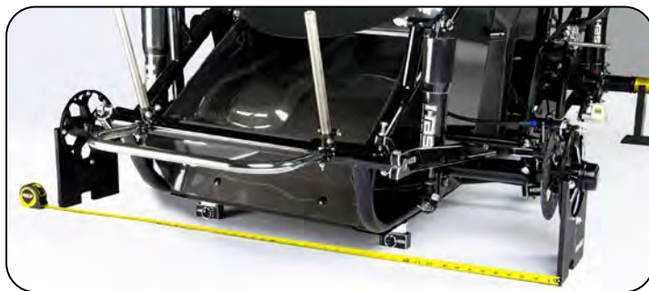
The car will now be resting on the blocks and the axles will be held up by the front plates and the rear squaring blocks.
