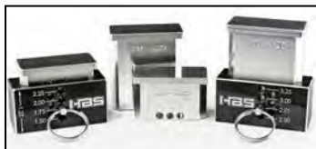
Set-Up Blocks are adjustable from 1" to 3 1/4" at 1/4" increments with many 1/8" increments. 1 5/8", 1 7/8", 2 1/8", 2 5/8", 2 7/8", 3 1/8" heights are provided. CNC machined aluminum, anodized. Set-Up Blocks (set, as shown) 80-600 $79.50
