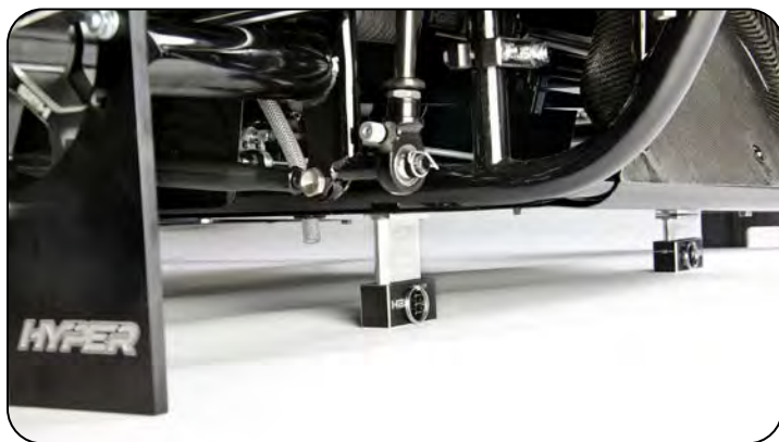
The car will now be resting on the blocks and the axles will be held up by the front plates and the rear squaring blocks.
