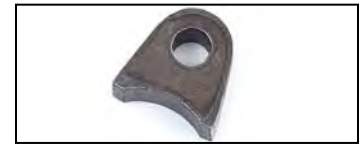
Top Jacob's Lower Tab 3/8" thick, 5/16" hole, 1-1/4" notch, 1/2" from center of hole to edge of notch. Used to go between the Jacob's ladder paddles on the bottom rail.
